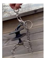
**Example** of a bit that is not with fixed mouthpiece (but limited in the looseness at the cheek/mouthpiece connection point - making them angle when doing the hanging test) and therefore ACCEPTED.
