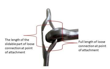
In case the curved sliding bar and the check connects in a very small slit, only the length of the slidable part of loose connection at point of attachment is measured (min. 1.5cm and max. 2.6cm).
